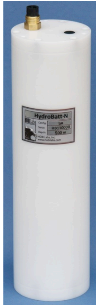
Figure 1. HydroBatt. The black circle opposite the connector on the top end cap is the pressure relief valve. Never block the valve. If it pops up, that indicates a possible hazard and you should discontinue use.
