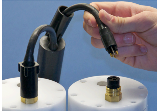
Figure 3. Beware of a short-circuit hazard in this situation: when one branch of the Y-cable is connected to a HydroBatt, the male pins of the other branch carry the first battery's output voltage!
