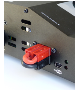
Figure 6. This connector is required for the charger to operate. Do not remove it.
