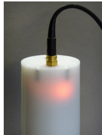
Figure 7. A red light inside the battery indicates it is blocking charge current because of excessive temperature
